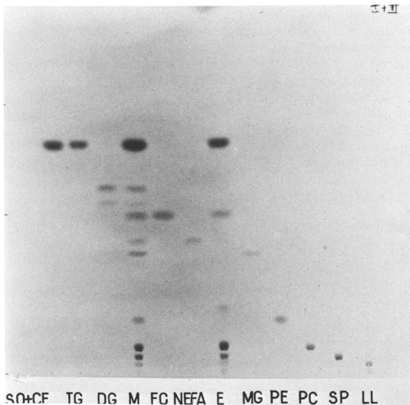
Fig. 1. Thin-layer chromatogram of lipids developed in solvent systems I + II. SQ = Squalene; CE = cholesterol ester; TG = triglycerides; DG = diglycerides (diglyceride 1,3 = 1,3DG and diglyceride 1,2 = 1,2DG); M = reference mixture of the twelve standard lipids; FC = free cholesterol; NEFA = non-esterified fatty acid; E = human serum lipid extract; MG = monoglyceride; PE = phosphatidyl ethanolamine; PC = phosphatidyl choline; SP = sphingomyelin; LL = lysolecithin.
